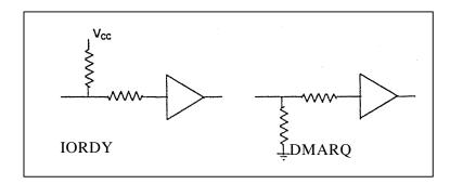
Figure 5.9 Ultra DMA termination with pull-up or pull-down
